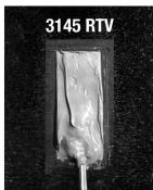
Quality of the bond often can be improved by applying an appropriate primer to chemically activate the specimen surface. (Micro-Measurements offers RTV Primer No. 1, which can be used on a wide variety of materials.) However, if the surface is properly cleaned for gage bonding (and is not re-contaminated during gage installation), the application of a primer is often unnecessary.
